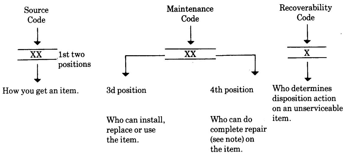
\*Complete Repair: Maintenance capacity, capability, and authority to perform all the corrective maintenance tasks of the "Repair" function in a use/user environment in order to restore serviceability to a failed item.
